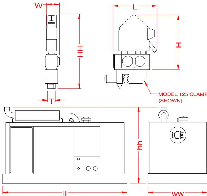
2. MODEL 223 VIBRATOR (with hydraulic clamp)
